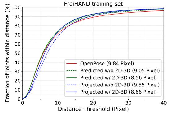
**Figure 4:** A comparison of 2D keypoint sets used or outputted at the training stage on FreiHAND. The fraction of joints within distance is plotted. The average 2D distances in *pixel* are shown in the legend. Refer to Section 4.4.2 for details.
