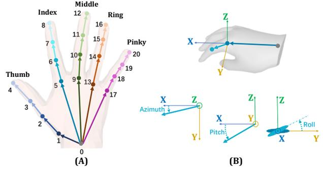
**Figure 3:** (A) Joint skeleton structure. (B) A sample of bone rotation angles. The five bones  $(\vec{01}, \vec{02}, \vec{09}, \vec{013}, \vec{017})$  on the palm are fixed. Each finger has 3 bones, and the relative orientation of each bone from its root bone is represented by azimuth, pitch, and roll.
