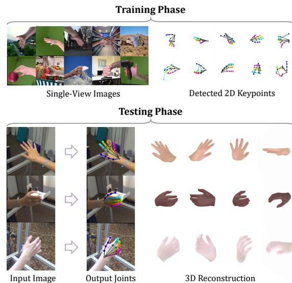
**Figure 1:** Given a collection of unlabeled hand images, we learn a 3D hand reconstruction network in a self-supervised manner. Top: the training uses a collection of unlabeled hand images and their corresponding noisy detected 2D keypoints. Bottom: our model outputs accurate hand joints and shapes, as well as vivid textures.
